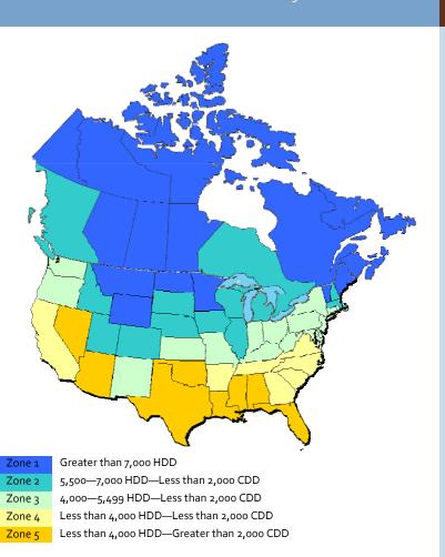
The benefits of insulation vary with the climate and are generally more pronounced in colder regions where significant energy is used to heat a home. A common method used to distinguish climate zones in North America is by measuring a region's Heating Degree Days (HDD) and Cooling Degree Days (CDD) using a base temperature of 65°F. The annual HDD for a region is the sum of the daily differences between 65° and the average daily temperature (ADT) when it falls below that target.
