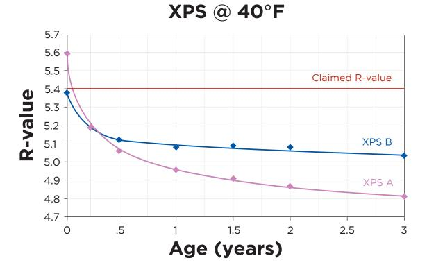
XPS manufacturers publish an R-value of 5.4 at a mean temperature of 40°F. The data shows performance below the published R-value of 5.4 for both of the manufacturers within 1 month after the samples were obtained.
