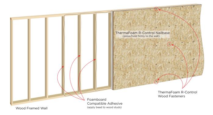
**Notice:** ThermaFoam R-Control insulation contains a flame retardant; however, it should be considered combustible and should not be exposed to sources of ignition. The product will ignite when exposed to open flame or welding torches.
