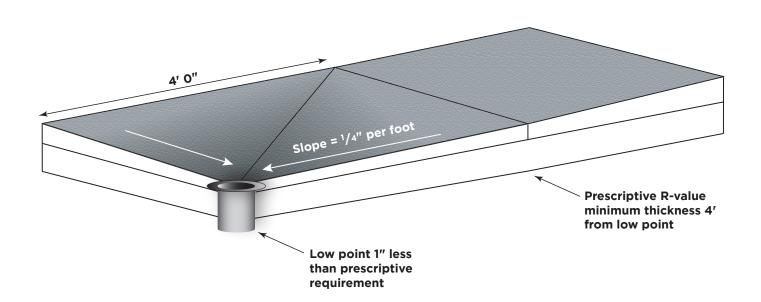
The table included with this bulletin provides the minimum prescriptive insulation requirements of IECC-2015. Alternative paths for conformance through detailed analysis are also available within the standard. Insulation requirements vary according to Climate Zone.
