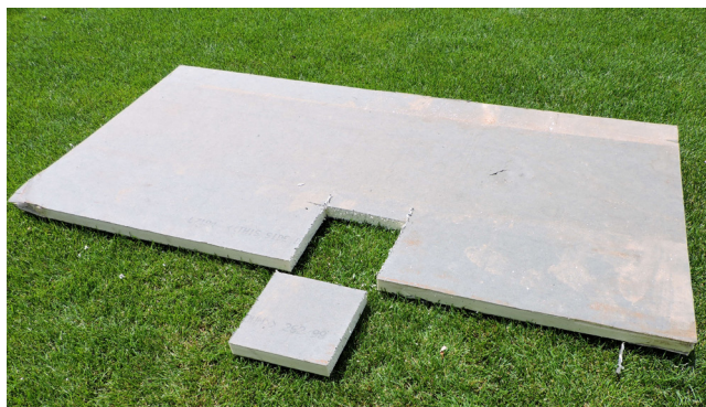
Figure 5. 17 year old polyiso sample
