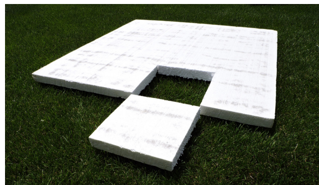
Figure 6. 17 year old Molded polystyrene sample
